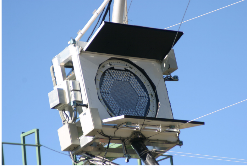
Figure 5.12: Picture of the camera of the MAGIC telescope. The two different regions –smaller pixels in the inner region and larger ones in the outer rings– can be clearly distinguished.
