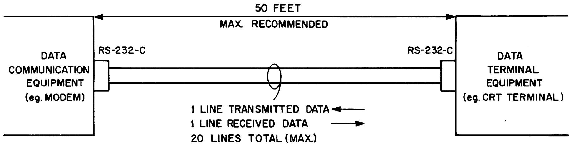
FIG. 3 - RS-232-C SERIAL INTERFACE STANDARD
