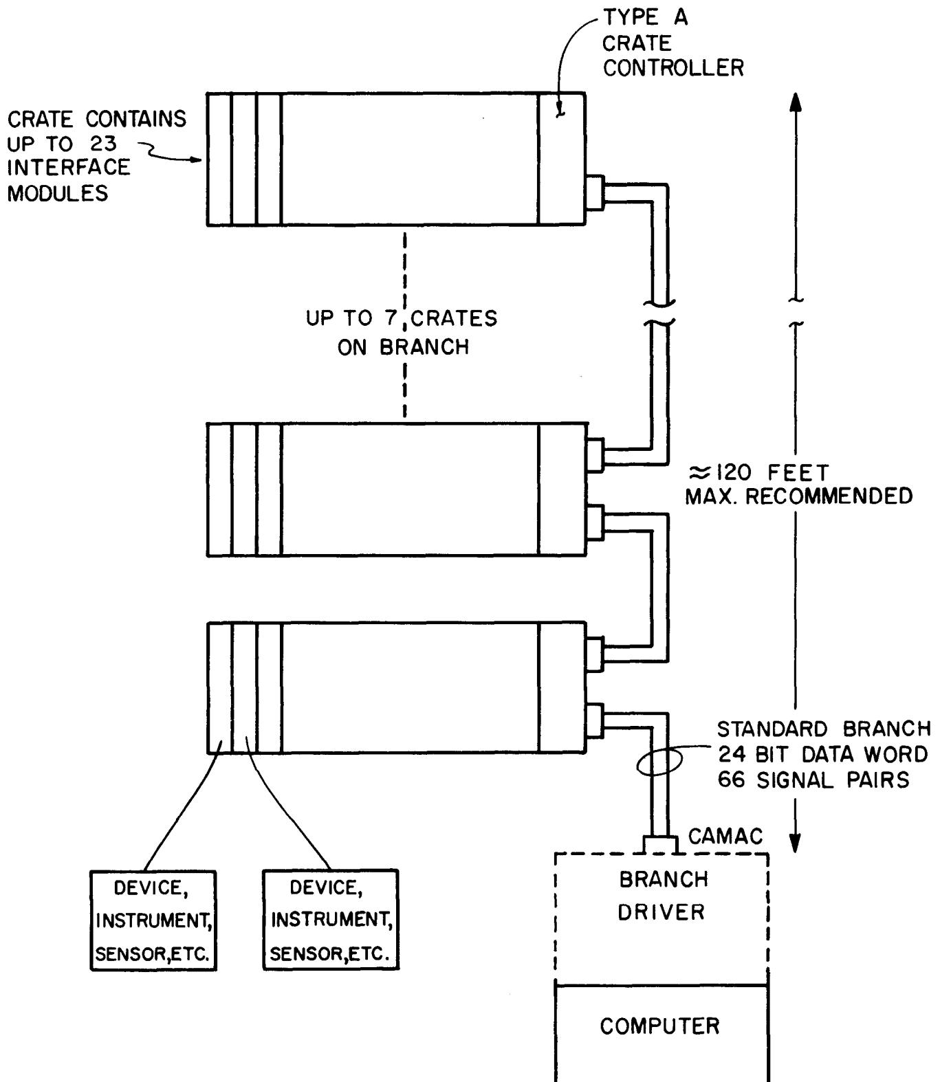
FIG. 4 - CAMAC STANDARD-PARALLEL BRANCH
