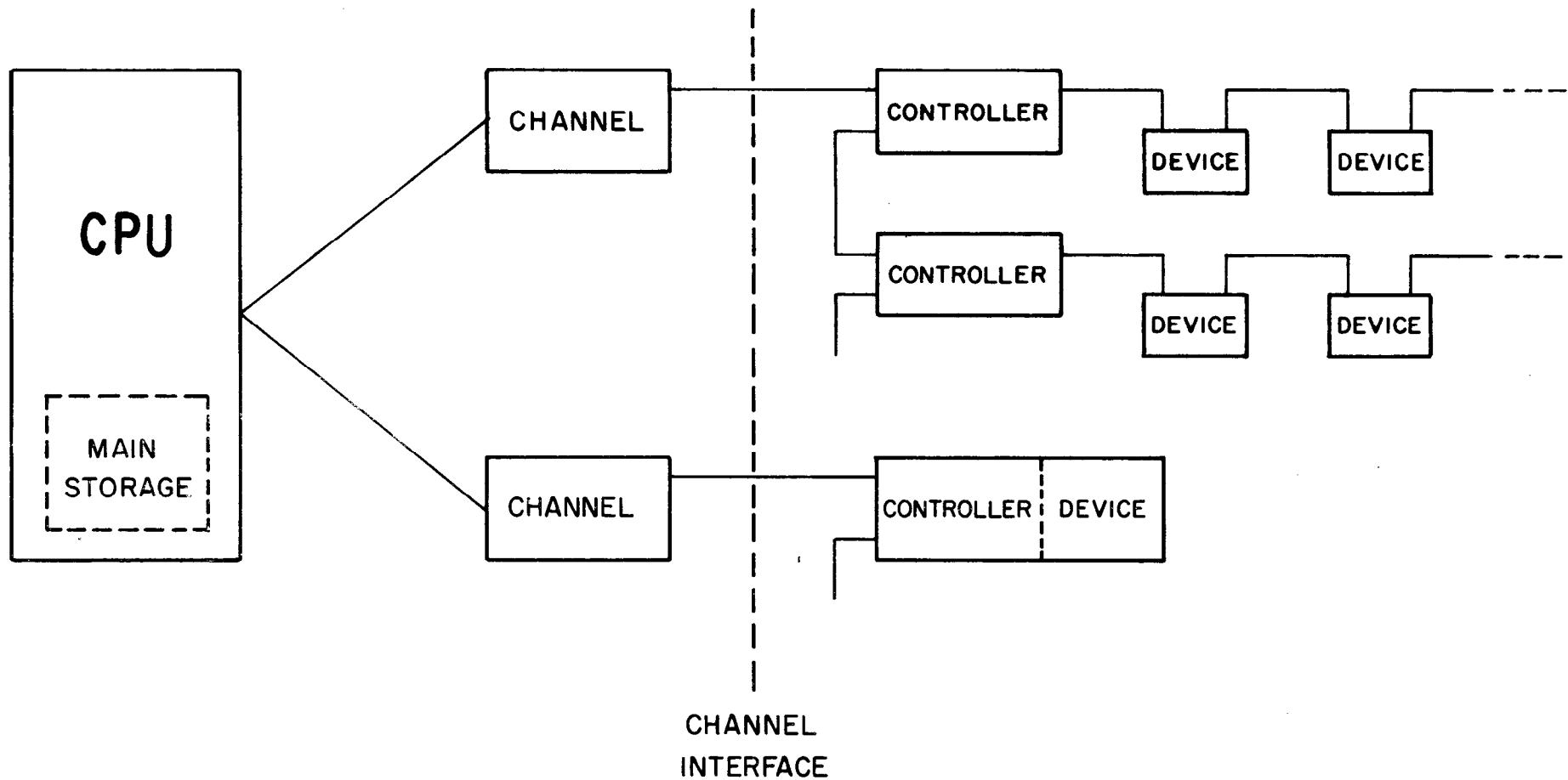
FIG. 5 – CHANNEL LEVEL INTERFACE
