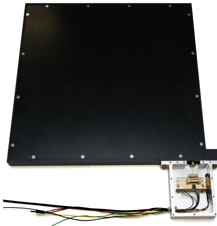
Figure 8.7.: The AMD tile container with opened SiPM compartment. One AMD scintillator tile is enclosed in the flat light-tight black box. One SiPM and temperature sensor is placed in the attached aluminum box (also light-tight during normal operation).
