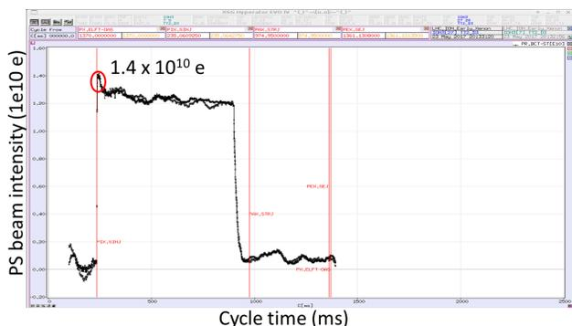
Figure 3: First circulating xenon beam in PS. Initial injected intensities  $\approx 1.4 \times 10^{10} e$ .
