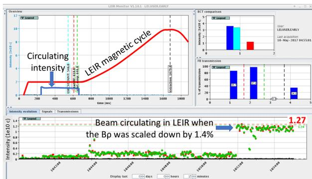
Figure 2: First circulating xenon beam in LEIR.
