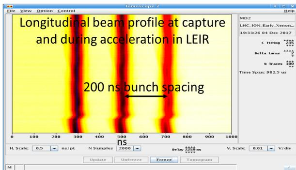
Figure 5:  $h=3+6$  in LEIR at 200 ns bunch spacing. The three bunches are transferred to PS where, after acceleration, they are compressed to 75 ns.
