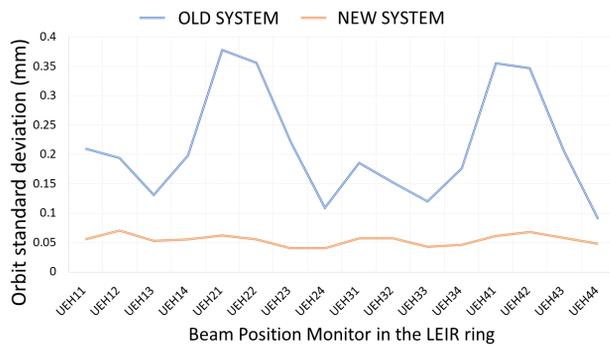
Figure 4: Comparison of the standard deviation measured by the old and new LEIR orbit acquisition system.
