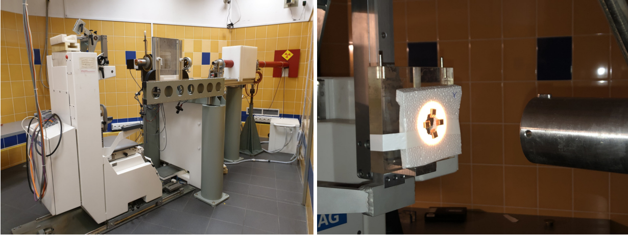
Figure 6.9: Left: Irradiation setup at IFJ-PAN, Krakow, Poland. Right: Four single channel SiPMs placed on the proton beam axis (taken from [51], with permission).
