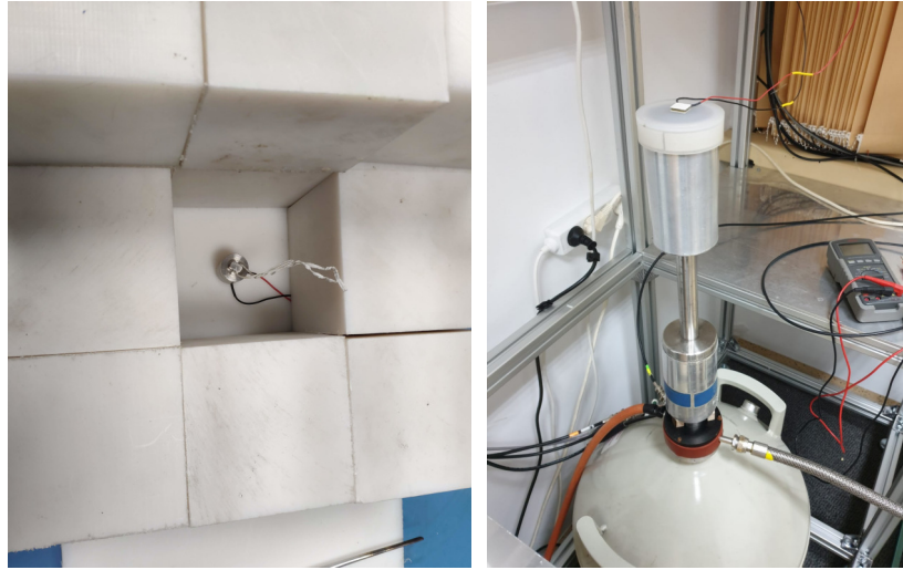
Figure 5.16: Left: PuBe source placed directly on top of the Peltier element, surrounded by 10 \times 10 \times 10 \text{ cm}^3 boronated cubes of polyethylene for neutron shielding. Right: Peltier element placed on a HPGe detector for activation measurement.
