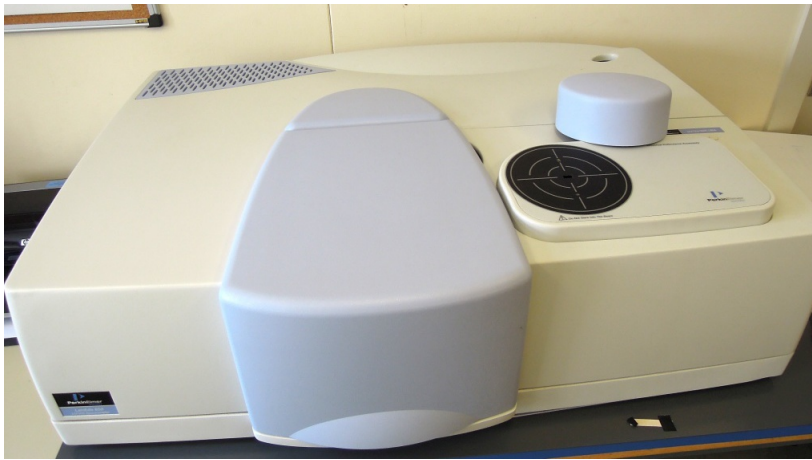
Figure 7.2: Perkin Elmer Lambda650 Spectrometer equipped with the Universal Reflectance Accessory used to measure the specular reflectance
