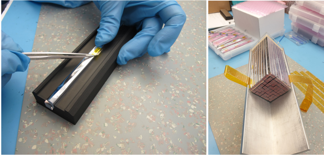
Figure 5.8: Left: Wrapping of a POLAR-2 scintillator bar [53]. Right: Fully wrapped target being assembled in the plastic alignment grid [53].
