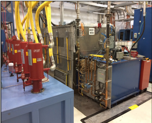
Figure 4: Prototype PPU HVCM during a heat run.
