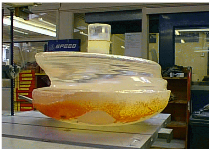
Figure 3-4. Example of a boule which suffers from moderate “tilt”; a region in which undercutting has occurred during crystal growth is clearly shown on the left-hand side of the boule.
