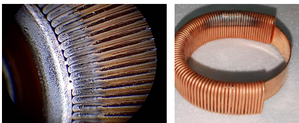
Figure 4: Observed damages at the cathode spring region: in-situ observation (left) and marks at the dismounted spring (right).
