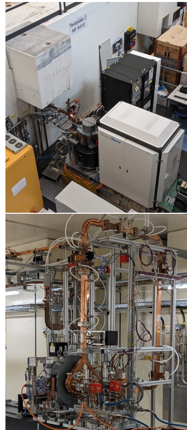
Figure 1: High power klystron-modulator (Top) and installed SW RF Photogun in test stand (Bottom).
