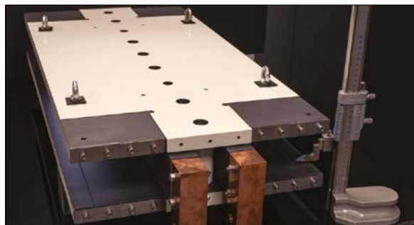
Fig. 2. Left: winding of the enhanced racetrack model coil (RMC) for FCC-hh 16T magnets with \text{Nb}_3\text{Sn} superconducting cable at CERN. Right: A 1 m-long prototype of the FCC-ee dipole magnet. The proposed design considerably reduces the power consumption and the total amount of material required. For example, a machine three times longer than LEP will only require around 35% more steel.
