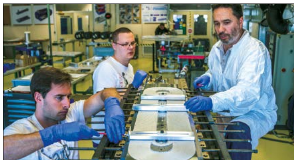
Fig. 2. Left: winding of the enhanced racetrack model coil (RMC) for FCC-hh 16T magnets with \text{Nb}_3\text{Sn} superconducting cable at CERN. Right: A 1 m-long prototype of the FCC-ee dipole magnet. The proposed design considerably reduces the power consumption and the total amount of material required. For example, a machine three times longer than LEP will only require around 35% more steel.
