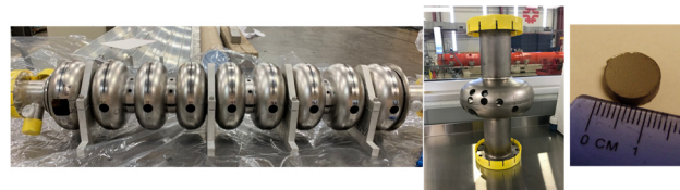
Figure 2: 9-cell 2/0 N doped cavity (left) with equator samples extracted from each cell. Single cell with cutouts from various locations and a typical sample is shown on the right.
