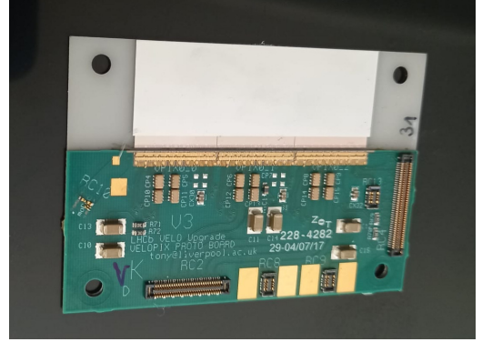
(b) Triple sensor bounded to the VeloPix.
