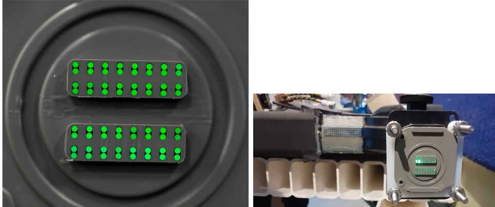
Figure 3.11: Optical connector consisting of WLS fibres from 32 cells. An unlit connector is shown on the left, on the right an opened extrusion (for demonstration purposes) is being manually lit up and the transported light illuminates the correct cell outputs on the optical connector. Left image courtesy of [84].
