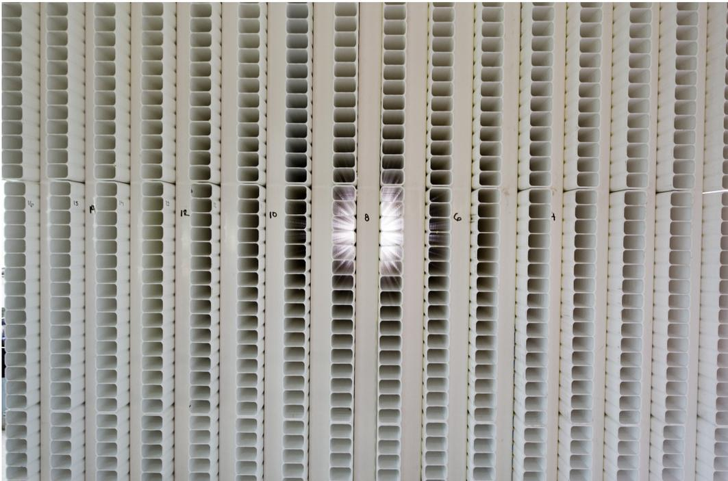
Figure 3.7: The bare PVC cells stacked in alternating planes to construct the frame of the NOvA detectors. Courtesy of [77].
