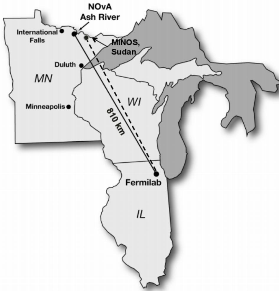
Figure 3.1: Map of the off-axis beamline originating at Fermilab. The near detector is located at Fermilab approximately one kilometer from the target, whereas the far detector is located 810 kilometers away at Ash River. Courtesy of [73].
