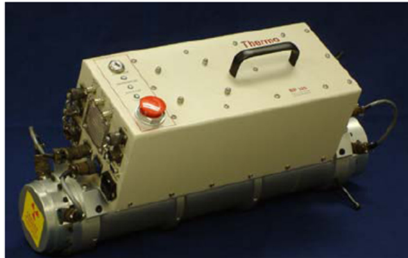
Figure 3.17: The neutron generator which is composed of an accelerating tube and an electronics part.
