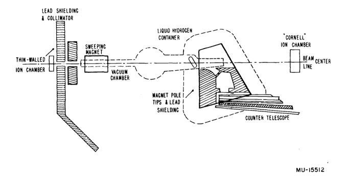
Fig. 1. Arrangement of experimental apparatus for small-angle measurements.
