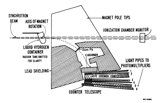
Fig. 9. Magnet and counter-telescope arrangement used in the angular range from 0° to 50°.
