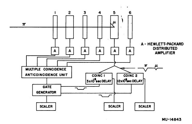
Fig. 3. Block diagram of  $\pi$  -  $\mu$  electronics.
