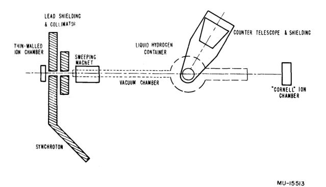
Fig. 2. Arrangement of experimental apparatus for wide-angle measurements.
