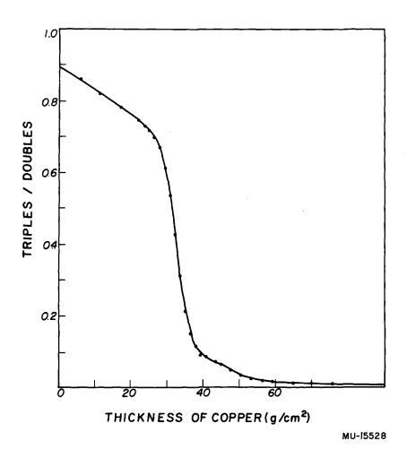
Fig. 22. Range curve in cyclotron pion beam.  $E_{\pi}$  = 87 Mev.
