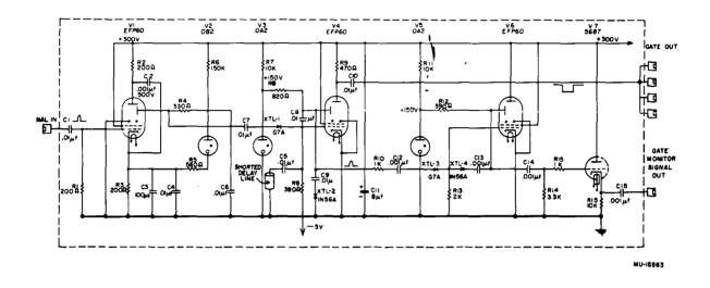
Fig. 4. Circuit diagram for gate generator.
