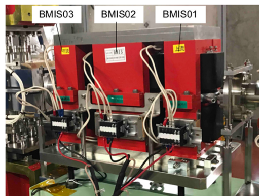
Figure 3: Chicane magnet installed in the cERL.
