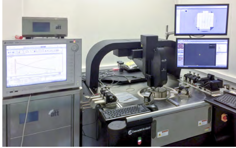
Figure 6.2: Semi-automatic probe station.
