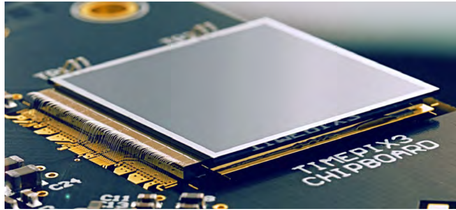
Figure 4.21: Picture of a silicon planar sensor bump-bonded to the Timepix3 ROC below, wire-bonded to the chip-carrier board [95].
