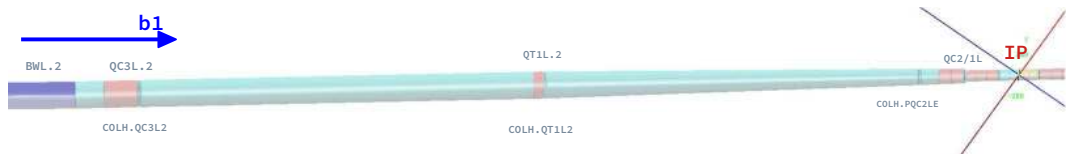
Figure 7.66: Top view on the updated geometry in Root display over the last 100 m upstream. Three collimators inserted after QC3L.2, QT1L and right at the entrance to the interaction region. The tapered beam-pipe downstream of QT1L is visible as well, indicating that COLH.PQC2LE needs a smaller aperture when completely opened than the other two collimators, which defaults to 35 mm.
