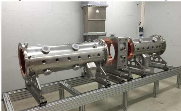
Figure 11: Prototype of coupled crossed-bar H-cavity.
