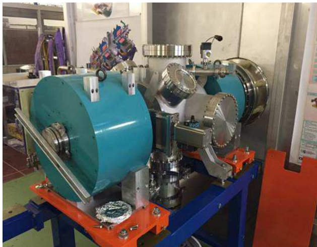
Figure 10: Proton source assembled at CEA/Saclay.
