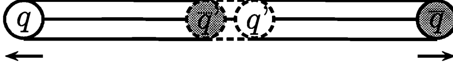
Figure 2.11: Description of color string stretched between a separating q\bar{q} pair. A string break is shown in the middle accompanied by the production of a new q\bar{q} pair.
