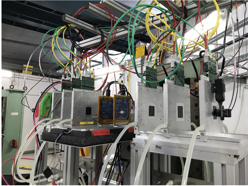
Figure 5.8 Photograph of the EUDET telescope at DESY with 6 MIMOSA26 planes and one DUT in the middle and a reference plane FE-I4 at the far end. This picture is taken on a different testbeam which had a different setup.
