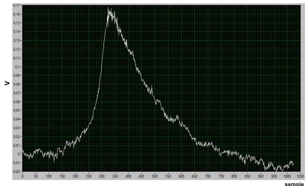
Figure 5. An event acquired during the 2022 data-taking period is shown: the peak-to-peak electronic noise corresponds to about 0.5 mV.
