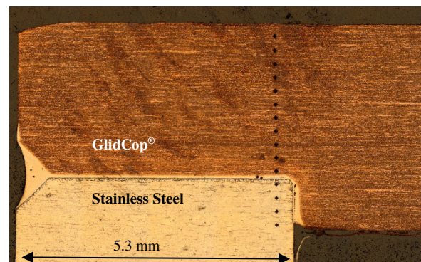
Figure 3: Stainless steel to GlidCop ® vacuum braze.
