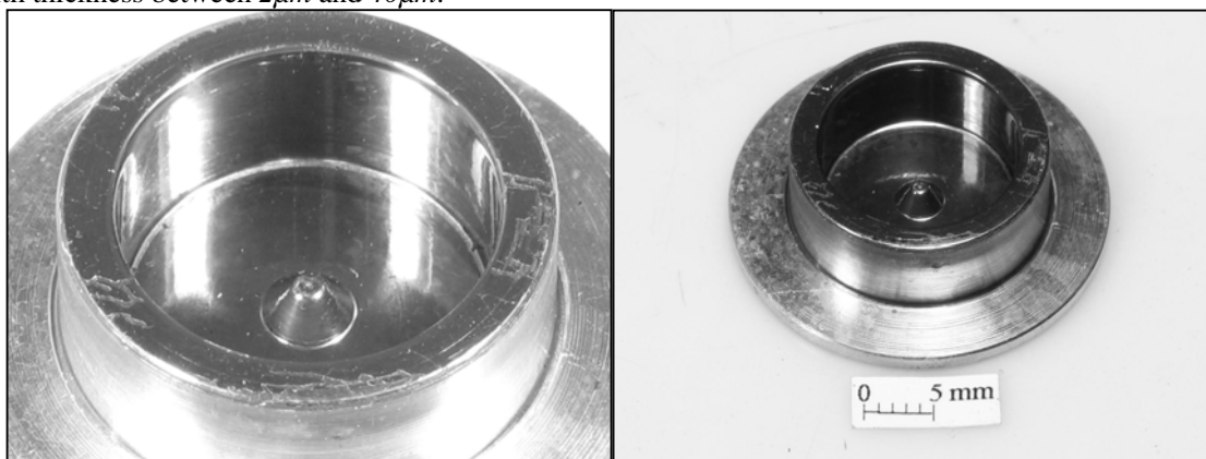
Figure 3 - Copper-aluminum klystron cavity covered with a thin layer of niobium.
