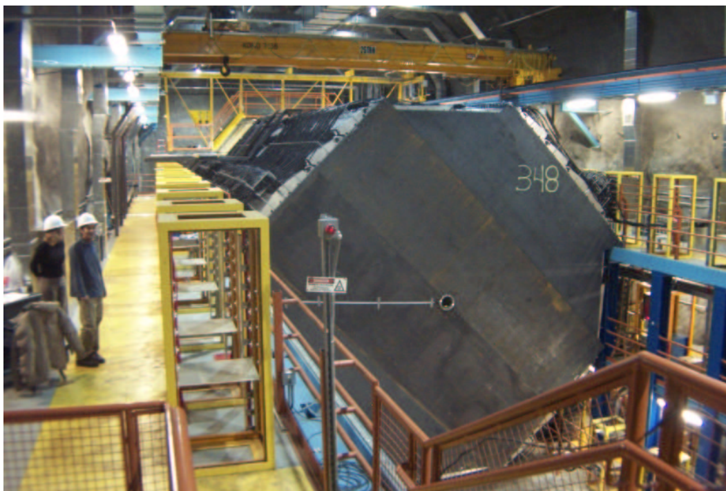
Figure 4.9: A photograph of the far detector during construction. The detector is built up to plane 348 at this point. The black conduit for the readout cables is clearly visible on the top left of the detector. Also the hole for the magnetic coil is present in the centre of the plane.
