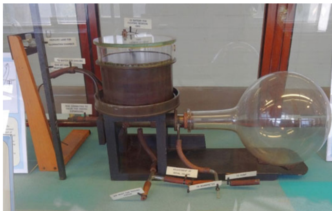
Fig. 5.6 Improved version of Wilson's chamber, 1911, exhibited at the Cavendish Museum. According to what Wilson himself reported, no other specimens of this chamber were built. Source Wikimedia Commons, Creative Commons Attribution-Share Alike 4.0 International License
