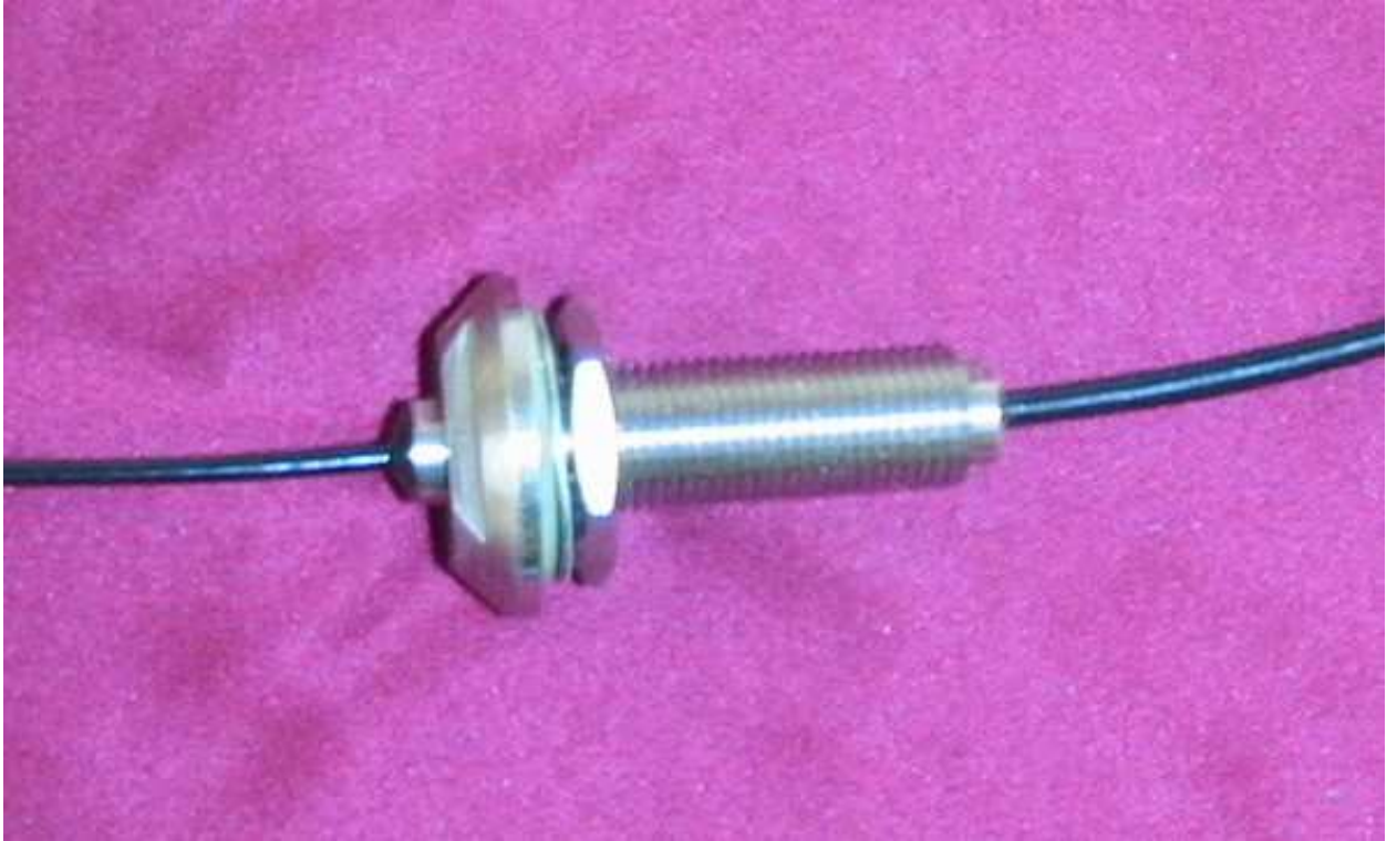
Figure 2.16: Photo of a vacuum fibre feedthrough.
