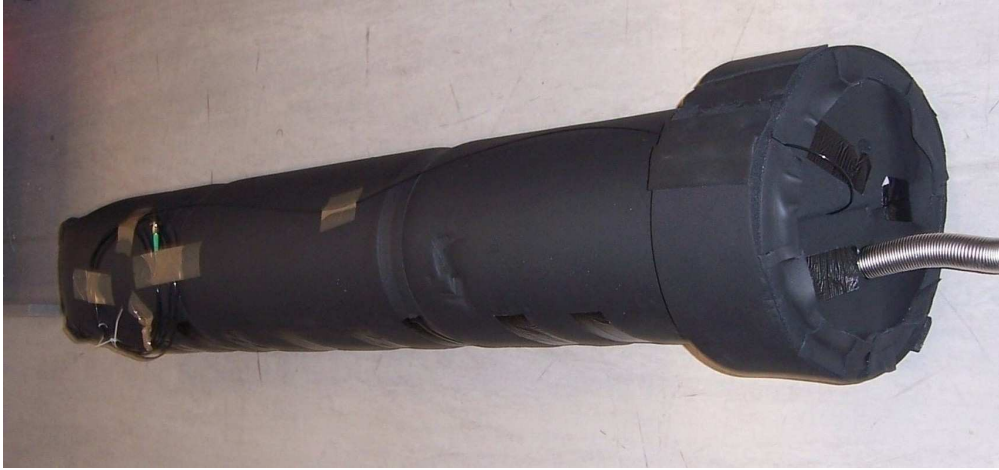
Figure 5.5: Photo of an insulated reference interferometer
