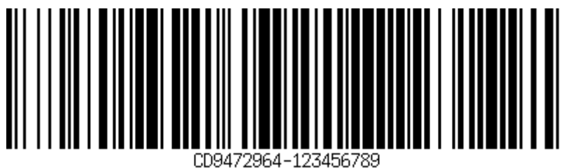
Figure 2: example of the custom barcode required on each system unit and enclosure. The first part before the dash ('-') is the CERN contract identifier and the second part is the vendor serial number. The same information must be burned into the FRU of the BMC of the system.
