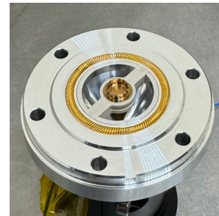
(b) EO-BPM button assembly, mating view
