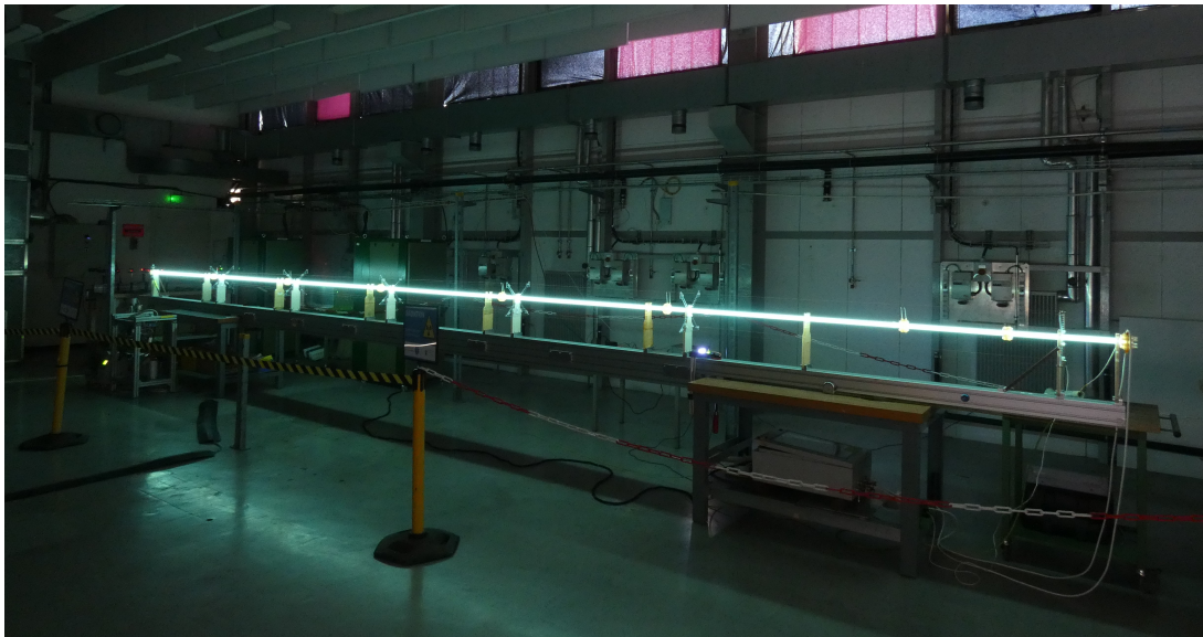
Figure 5.1: Plasma discharge in CERN DPS laboratory - Xe, p = 16 Pa, I_h = 500 A, I_{plasma} = 10 m
