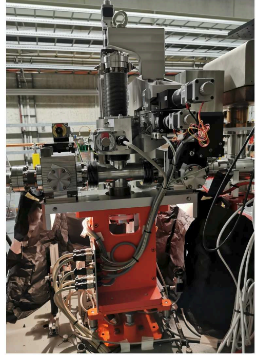
Figure 3. Installed collimator device. An adjustable support allows precision alignment to the beamline. Cameras observe the collimator position through window flanges from underneath. All collimators can be adjusted remotely.
