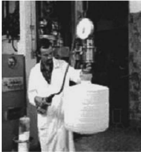
Fig. 5.19. Large-size halide scintillation single crystal ingot (Courtesy of Amcryst-H, Ltd)
