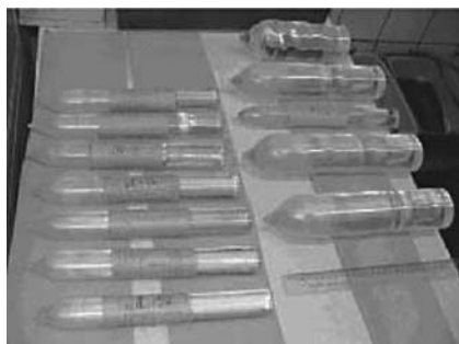
Fig. 5.22. PWO single crystal grown by the Czochralski method
