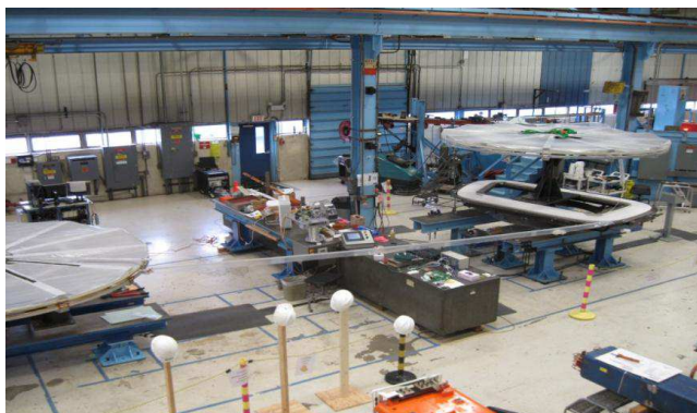
Fig. 5. Partial view of the coil fabrication shop at Fermilab showing a coil being wound, the second spool is seen above the winding table.
