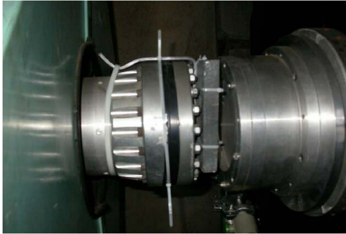
Fig. 6.8: The pre-shower fixed in between the last focusing magnet and the Cherenkov counter during the exposures.
