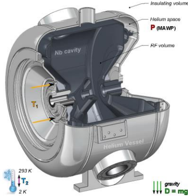
Fig. 9. Structural geometry of SSR1 with a cut showing the niobium bare cavity and the helium vessel.
