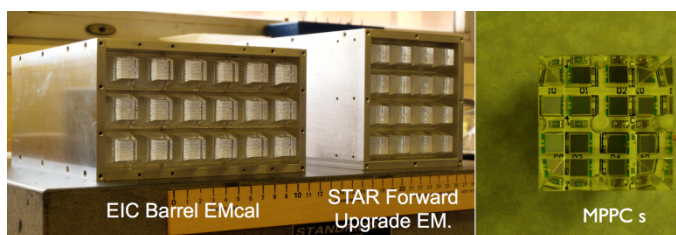
Fig 1. Two recent EM calorimeter prototypes built with our technique: an EIC barrel calorimeter with wedge-type towers and a prototype for the forward upgrade for STAR. Both were read out with silicon photomultipliers, shown on the right side.
