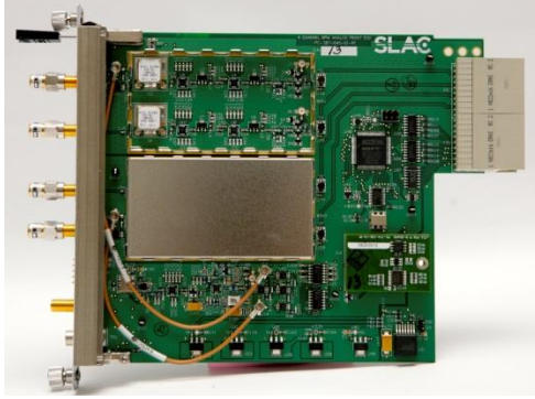
Figure 2: SLAC built BPM analog front end
