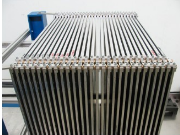
Figure 3.9: The tungsten absorber stack. It consists of 1 cm thick tungsten plates where the active layers are mounted in between.
