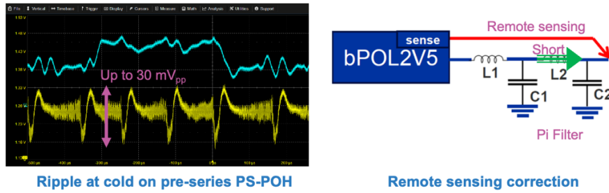
Figure 6. BPOL2V5 cold oscillations and correction of the remote sensing scheme.
