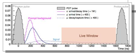
Fermilab accelerator complex provides ideal pulse spacing for Mu2e. Suppress prompt backgrounds by many orders of magnitused beam allows to suppress prompt background during proton-pulses be Must achieve extinction  $Q_p^{1/2}$  out of the bunch)  $(N_p^{-1})$  in bunch)  $\leq 10^{-10}$
