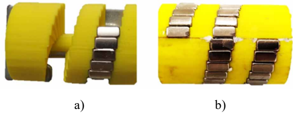
Figure 7: Assembly and axial magnetization of a two-period quasi-helix consisting of a spirally arranged set of 24 radially magnetized ring sectors per period. Magnetized sectors are glued into a mold placed on steel to weaken the forces of interaction between the magnets: a) the beginning and b) the end of the process.
