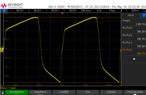
Figure 5: Module output voltages during a ramp (50V/div).
