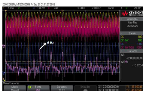
Figure 3: Measurements in laboratory for a 0 to 380 A ramp: Ch1: CB voltage (5V/div), Ch3: Load current (112.5A/div), Ch4: IS input current (5A/div), Math: Ch4 FFT (20dB and 2Hz/div).
