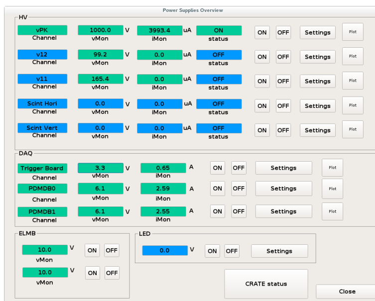
Figure 157: Overview of the values monitored by the power supplies. From this panel is also possible to control each channel and to show its current and voltage trending. Also the crate status can be monitored using the corresponding button.
