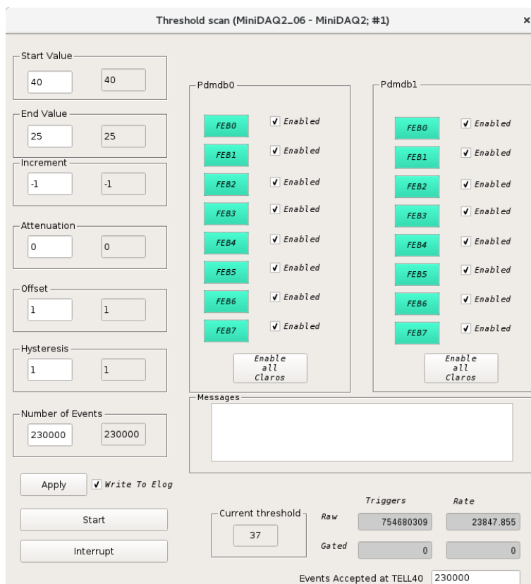
Figure 153: User interface used to perform threshold scans. The messages box shows message in case of errors during the run. The Write to Elog checkbox allows to send the DAC scans information to the LHCb RICH upgrade logbook for the inventory.
