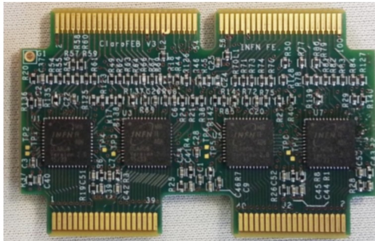
Figure 115: View of one side of a FEB, hosting four CLARO ASICs. The other four chips are hosted on the other side.
