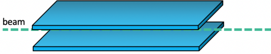
Figure 2.30: For the resistive wall contribution we suppose parallel plates with infinite thickness and use IW2D for the impedance and wakefield evaluation.
