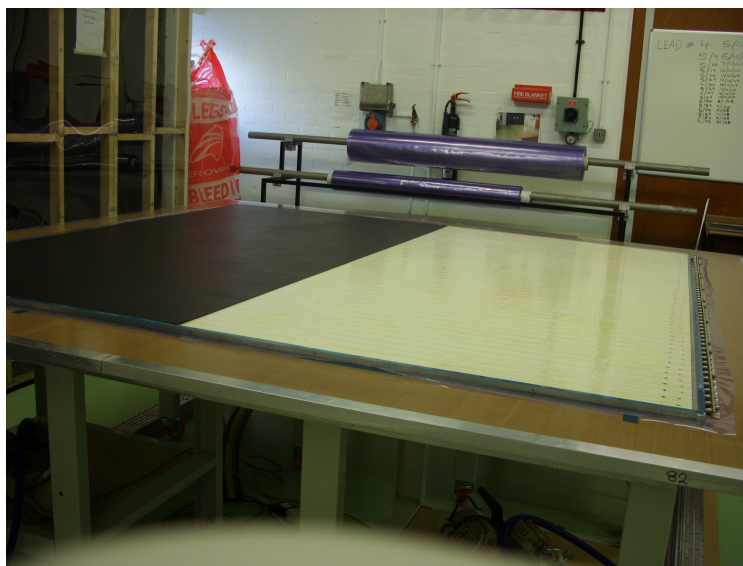
Fig. 4.5. Picture of a partially complete DS-ECal layer. One lead sheet has been glued to the scintillator bars. A second sheet is yet to be attached.
