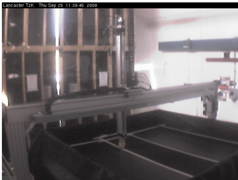
Fig. 6.2. The DS-ECal module is being scanned. The DS-ECal is made light-tight by a complete blackout material coverage. The horizontal arm above the centre of the layer is the scanner arm. The vertical arm attached to it holds the source, visible just above the surface of the layer. One can clearly see where tape is deployed to secure the blackout material.
