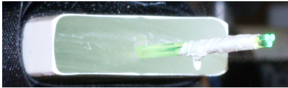
Fig. 5.3. Picture of the scintillator bar end with 3 WLS fibres for readout. Due to the elliptical shape of the hole it was possible to put 3 fibres down the central hole. The fibre ends are polished to an optical finish for coupling to the PMT. The fibres are held together with Teflon tape.
