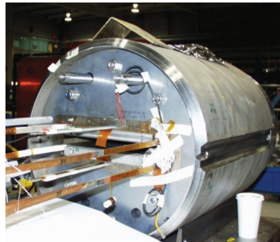
Figure 4: 10 T Nb 3 Sn common coil dipole DCC017 with a large open space for testing insert coil(s).
