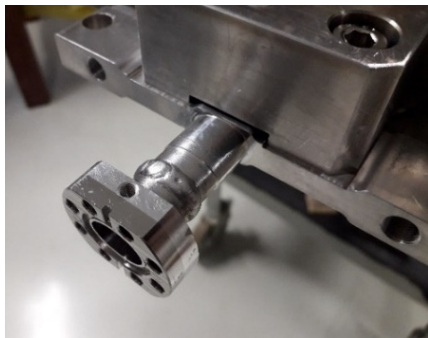
Figure 8: Vacuum flange welded to the chamber.
