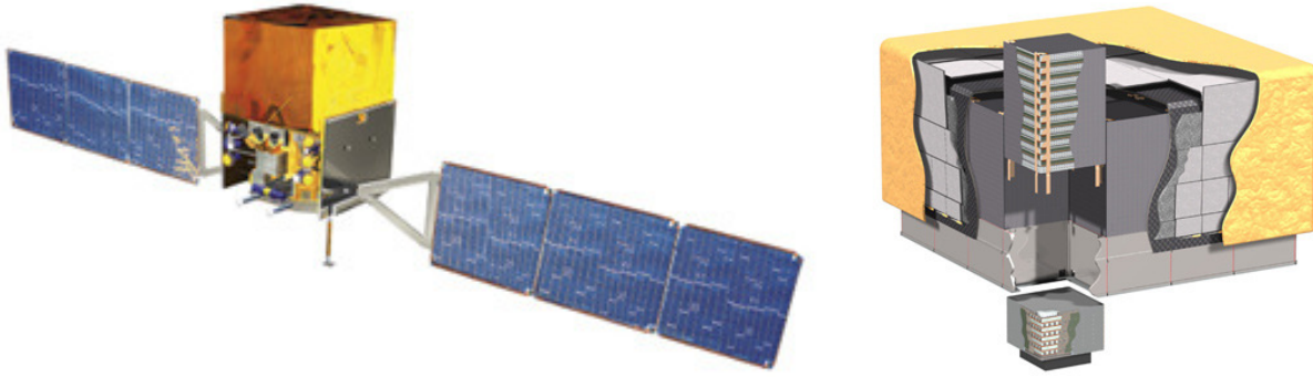
Figure 2.4.: Schematic diagram of the Fermi Gamma-ray Space Telescope (left) and detailed close-up view of the Large Area Telescope (LAT, right, see Sect. 2.2.1) showing one of 16 towers covered by the anti-coincidence shield to reject the charged cosmic particle background. Each tower consists of a converter, a calorimeter and a data acquisition module (Credit: NASA).
