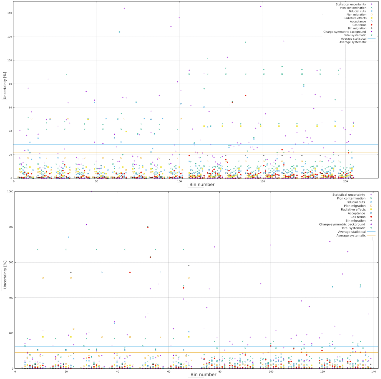
Figure 3.133: Contributions from different sources to the total relative uncertainty in the fully multidimensional binning for K^+ (top) and for K^- (bottom)
