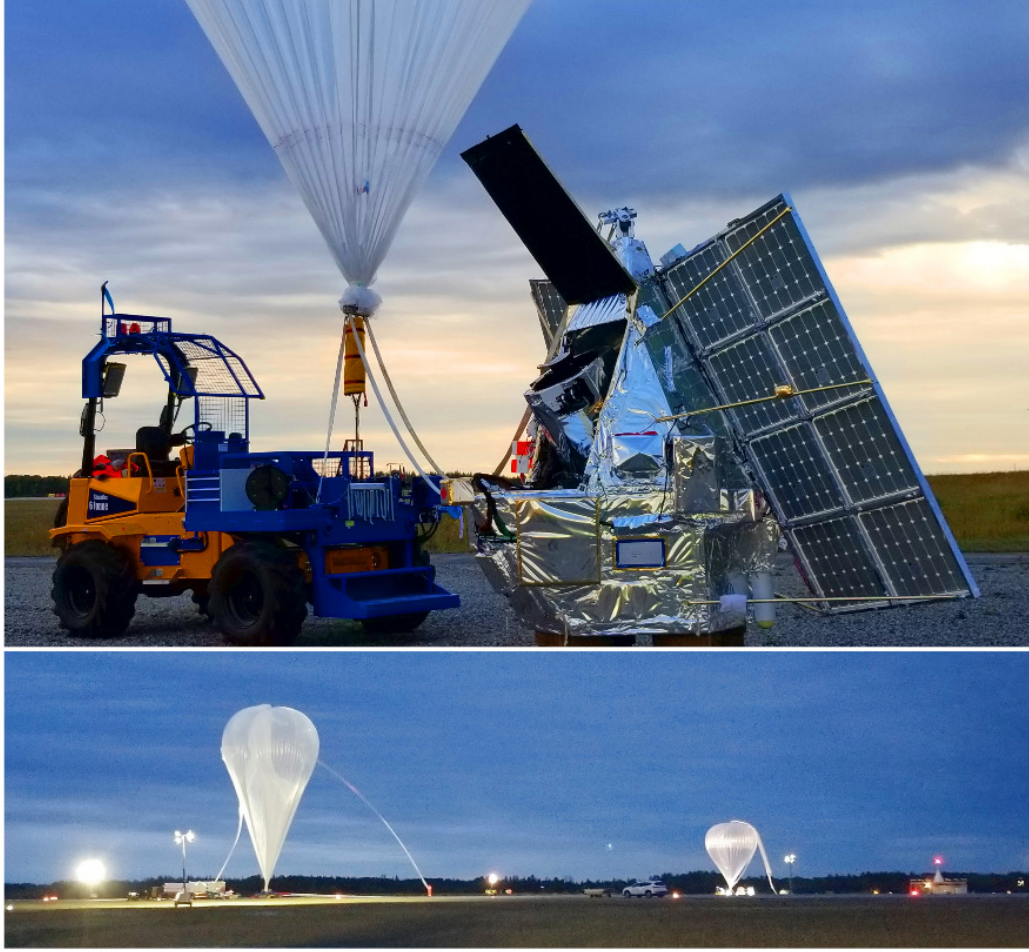
Figure 4.6: Figure 3 of Romualdez et al. (2020) . SUPERBIT just before the 2019 engineering launch. Top panel: the telescope is secured by a launch support vehicle beneath the tow balloon. Bottom panel: the telescope seen from a distance with both the tow (right) and primary (left) balloon. The smaller tow balloon provides neutral buoyancy for launch and is secured during inflation of the primary balloon.
