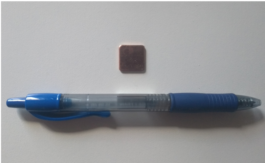
Figure 5.12: A copper heatsink that will be added directly to the processor chip of the Raspberry Pis. The pen is shown for scale.
